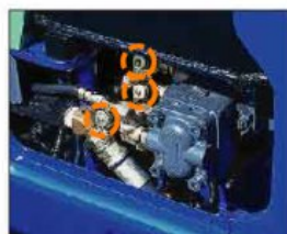
Oil pressure measurement port with coupler
