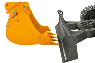
Close distance between Bucket Tooth and Dozer Blade
