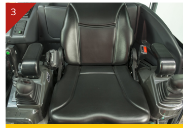
Full suspension seat - c/w retracting seat belt
