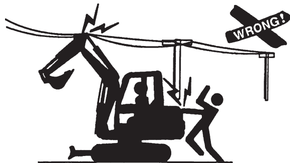
Electrical shock / electrocution
